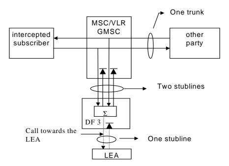
Figure 15: A two stubline configuration to DF3 for the interception of a circuit switched speech call
