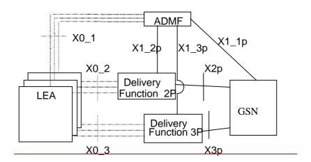
Figure B.1: Reference configuration for GPRS
