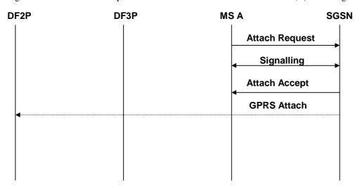
Figure B15: Interception of mobile originated GPRS attachment
